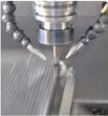
Figure 2: End milling with QuadCoatings Tools: Solid carbide end mills - d=8 mm - z=4 - a p =5 mm - a e =3.5 mm - v c =110 m/min - f=0.24 mm/rev Work piece material: DIN I.2085 - X33CrS16 - 31 HRC - External minimum lubrication.
